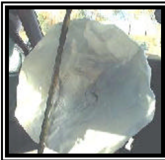
Figure 4. 1998 Jeep Cherokee redesigned driver air bag.
