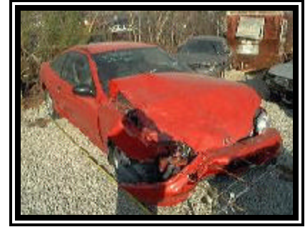
Figure 3. Front right damage to the 1998 Chevrolet Cavalier 2-door coupe.
