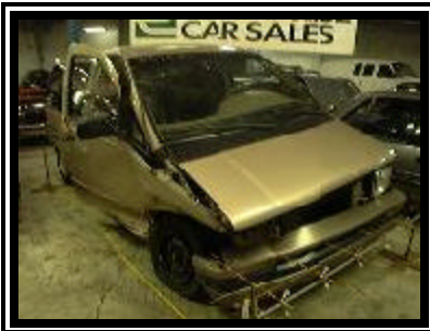
Figure 4. Front right damage to the 1992 Ford Aerostar minivan.
