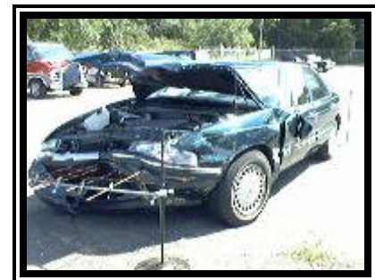
Figure 3. Frontal damage to the 1998 Buick LeSabre Limited.
