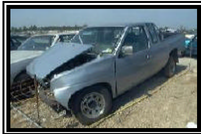
Figure 4. Frontal damage to the 1991 Nissan pickup truck.
