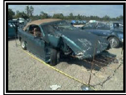
Figure 3. Frontal damage to the 1998 Ford Mustang convertible.
