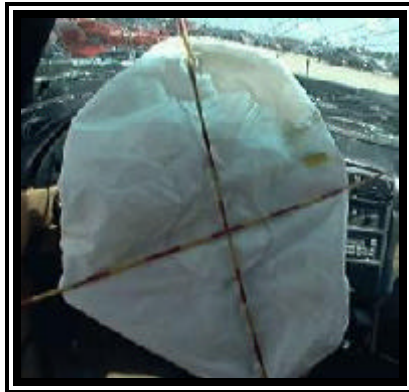
Figure 5. 1998 Ford Mustang redesigned driver air bag.
