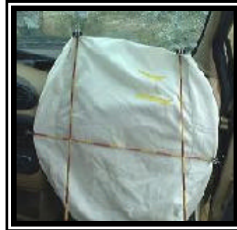
Figure 11. 1998 Plymouth Grand Voyager redesigned passenger air bag.
