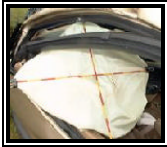
Figure 10. 1998 Plymouth Grand Voyager redesigned driver air bag.
