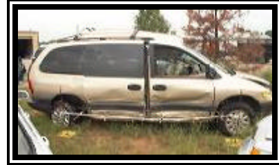
Figure 4. Right side damage to the 1998 Plymouth Grand Voyager.
