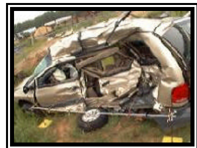
Figure 6. Left side damage to the 1998 Plymouth Grand Voyager.
