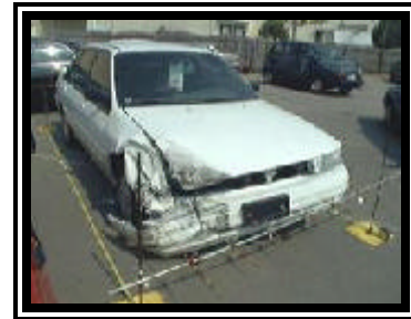
Figure 5. Frontal damage to the 1995 Ford Escort LX.
