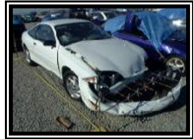
Figure 3. Frontal damage to the 1998 Chevrolet Cavalier.
