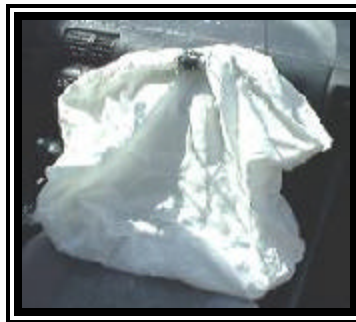
Figure 6. 1998 Saturn SL2 redesigned passenger air bag.
