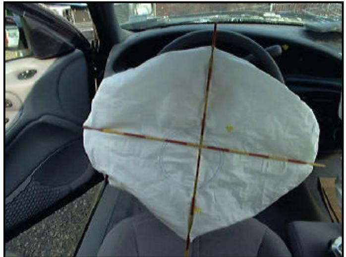
**Figure 5. Driver side air bag - Vehicle 1**
