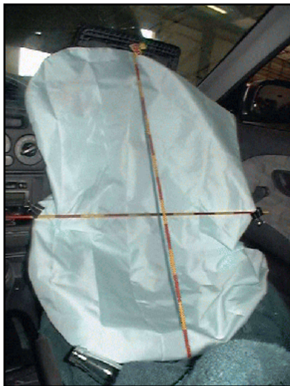
Figure 6. Interior, Vehicle 2, passenger's side redesigned air bag
