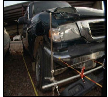
Figure 7. Close-up view showing right front bumper impact to case vehicle
