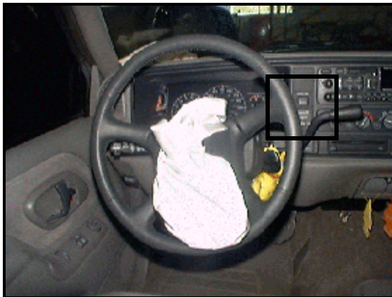
Figure 7. Interior, case vehicle. Box indicates location of air bag shut off switch.
