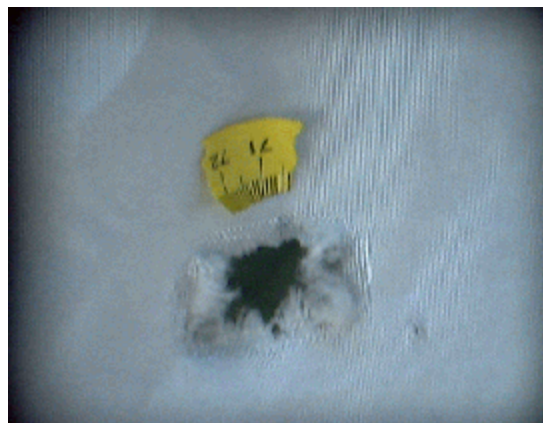
Figure 8. Passenger's side air bag damage
