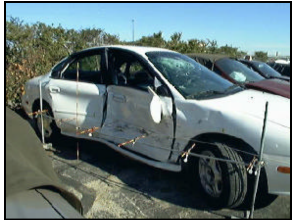
Figure 7. Close-up Showing Right Side Impact to Vehicle 1
