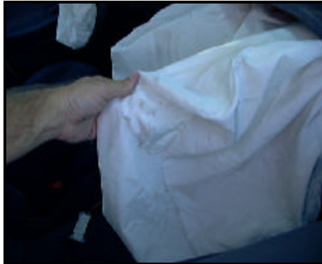
Figure 10. Right lateral views of passenger air bag showing small tears
