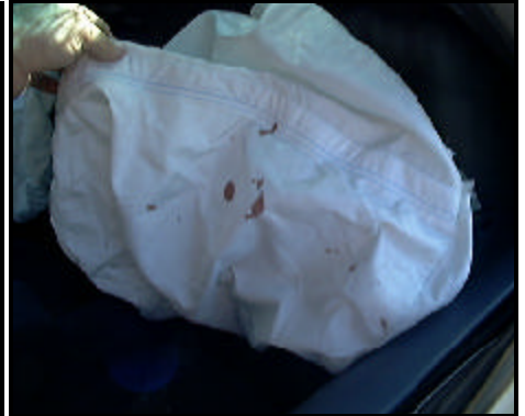
Figure 11. View of blood deposits to bottom of passenger air bag
