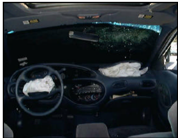
Figure 8. Interior of case vehicle showing drivers and passenger frontal air bags.
