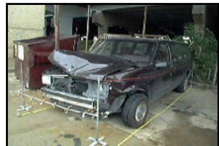
Figure 4. Frontal Damage to Vehicle 2
