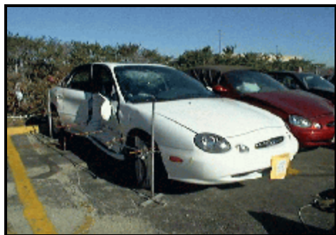
Figure 3. Right Side Damage to Vehicle 1
