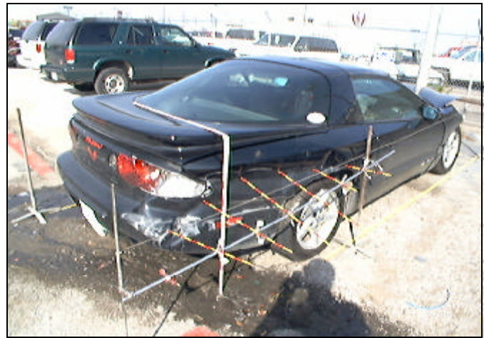
Figure 7. View Showing Secondary Right Quarter-Panel Impact to Firebird/Trans Am
