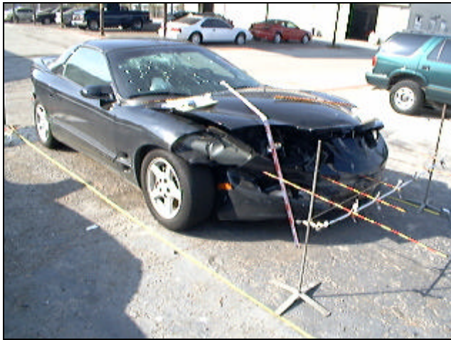
Figure 6. View Showing Initial Front Right Corner Impact, Vehicle 1 (1999 Firebird)
