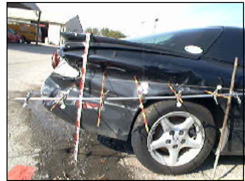
Figure 5. View Showing Secondary Guardrail Impact to Right Quarter-Panel
