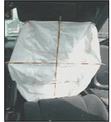
Figure 10. Deployed Passenger Air Bag
