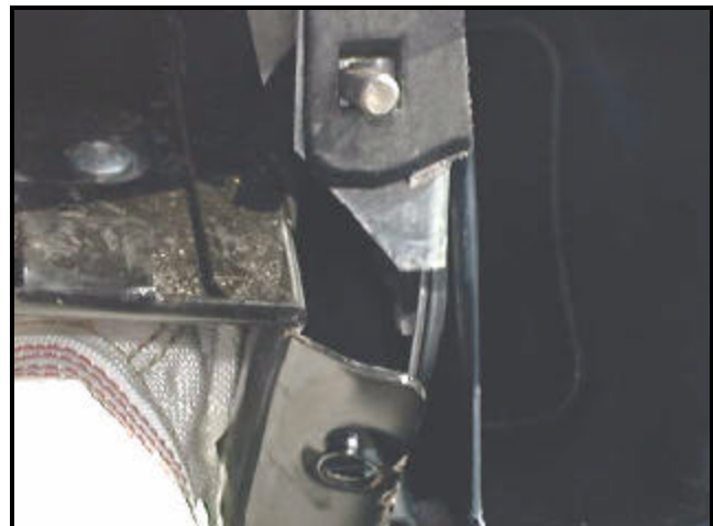
Figure 7. Passenger's frontal air bag. Close up of module retaining bolt failure.
