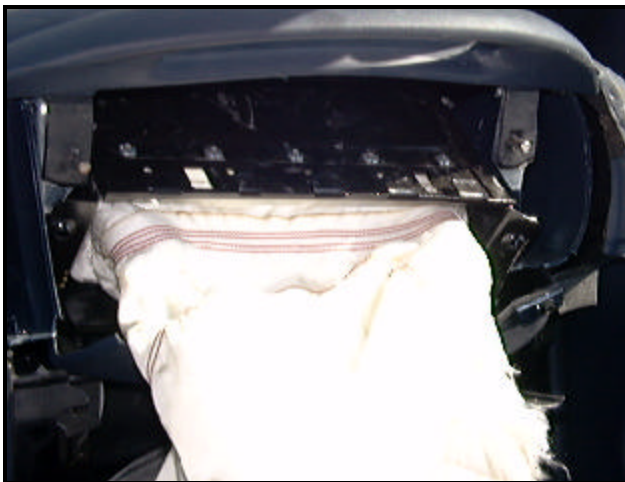
Figure 6. Passenger's frontal air bag. Module pulled out from instrument panel.
