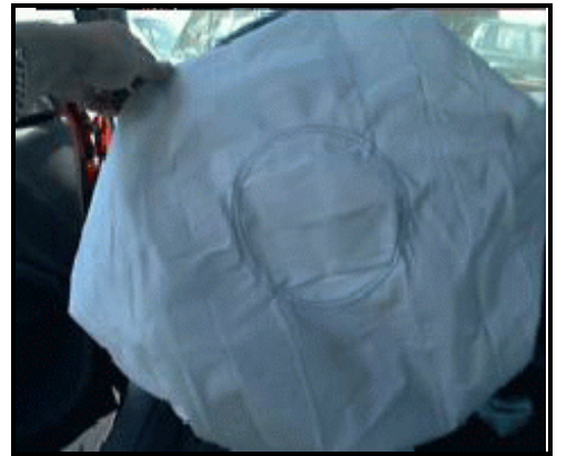
Figure 11. Deployed driver's air bag
