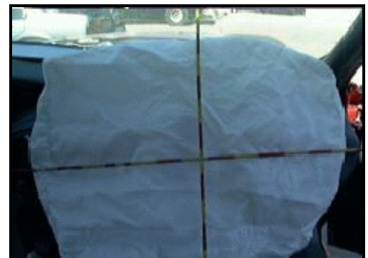
Figure 9. View showing the deployed passenger air bag
