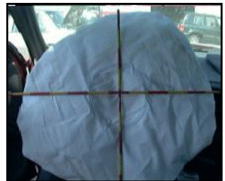
Figure 8. View showing the deployed driver's air bag
