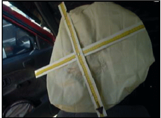
Figure 11. View showing deployed driver's air bag with lipstick transfer to upper right quadrant
