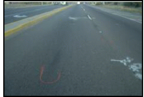
Figure 2. View showing pre-impact skidding from Vehicle 2
