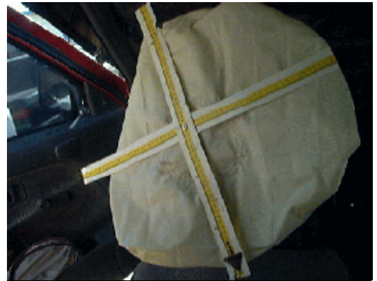
Figure 8. View showing deployed driver's air bag and lipstick transfer
