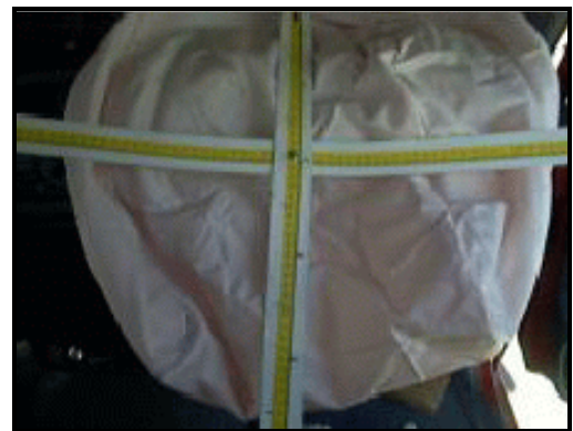
Figure 10. View showing deployed passenger air bag (lower half)
