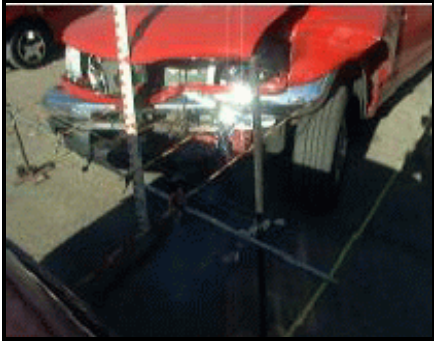
Figure 6. View showing frontal deformation to Vehicle 2
