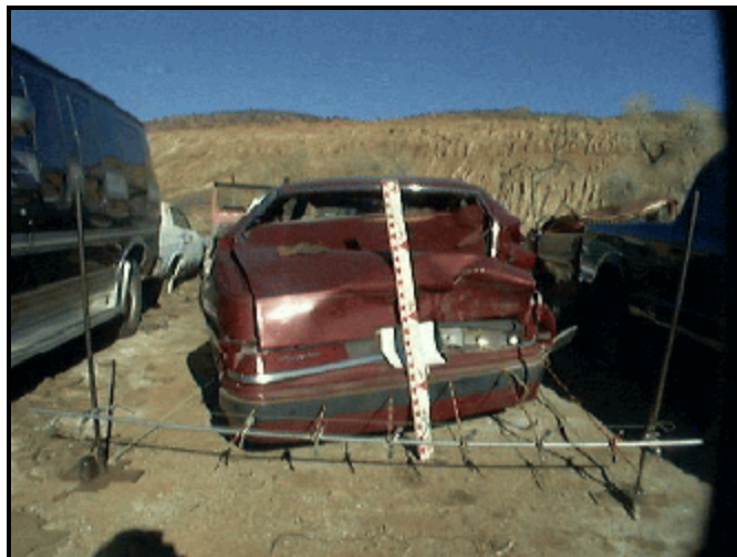
Figure 5. View showing damaged rear plane to Vehicle 1 (1986 Ford Thunderbird)
