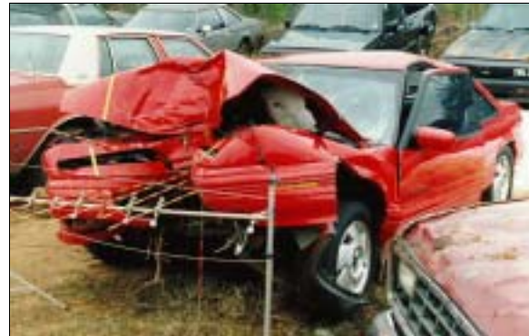
Figure 3: Case vehicle's frontal damage from tree impact, viewed from left of front with contour gauge present (case photo #13)
