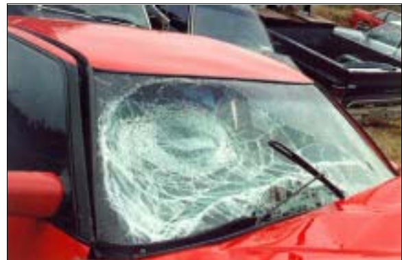
Figure 7: Right side of the case vehicle's windshield which was damaged by front right air bag module's tethered cover flap (case photo #20)
