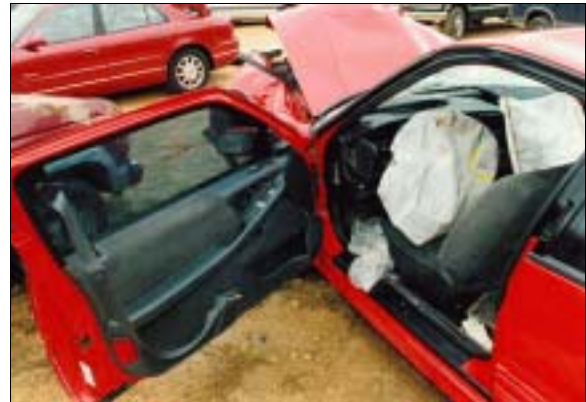
Figure 6: Case vehicle's driver seating area showing deployed driver and front right air bags; Note: three-point passive belt in driver's door (case photo #21)
