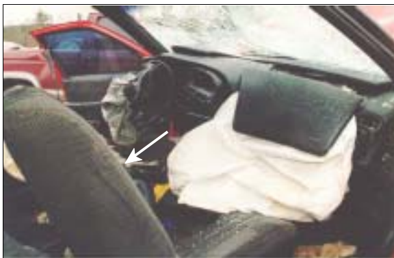
Figure 10: Case vehicle's front right passenger seating area showing deployed driver and front right air bags; Note: broken hinge (arrow) from center console's covered storage box and collapsed steering wheel rim (case photo #26)
