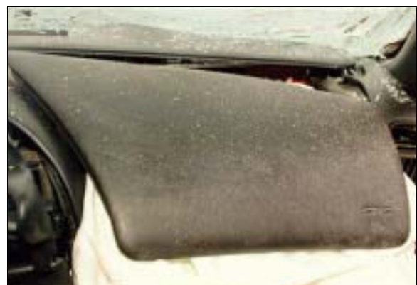
Figure 8: Case vehicle front right air bag module's tethered cover flap showing glass scratches from contacting and damaging right windshield (case photo #36)
