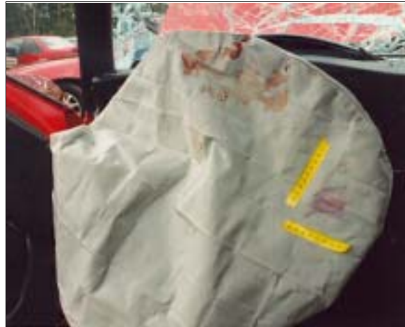
Figure 12: Close-up of case vehicle's driver air bag showing lipstick (i.e., upper right) and blood (i.e., upper center) smears (case photo #28)
