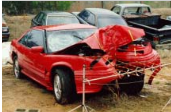
Figure 4: Case vehicle's frontal damage from tree impact, viewed from right of front with contour gauge present; Note: vertical yellow tape outlines direct contact area case photo #18)
