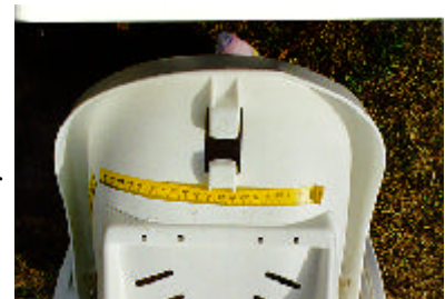
Figure 9. Cover flap abrasion and fracture to the shell of the child safety seat.
