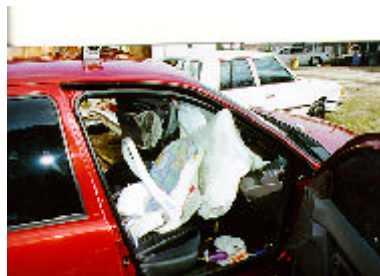
Figure 1. Expansion of the front right air bag against the shell of the infant restraint.
