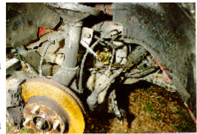
Figure 4. Undercarriage damage and separation of the left lower ball-joint.
