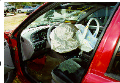
Figure 6. Deployed front left air bag.
