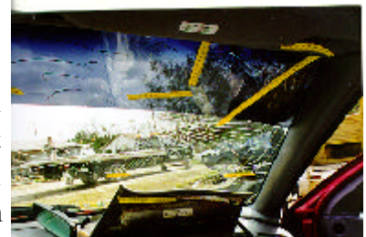
Figure 7. Cover flap and air bag contact to the windshield.
