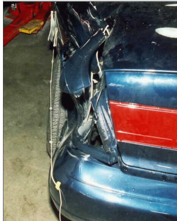
Figure 7: Case vehicle's side slap damage viewed from back along reference line (case photo #14)
