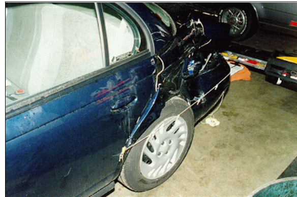
Figure 5: Case vehicle's side slap damage viewed from front of left (case photo #10)
