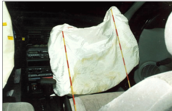
Figure 9: Case vehicle's deployed front right passenger air bag showing no obvious contact evidence (case photo #27)
