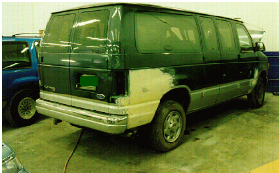
Figure 4: Ford's damaged right side showing primary impact to the right fender (replaced) and side slap impact to the right quarter panel (case photo #33)
