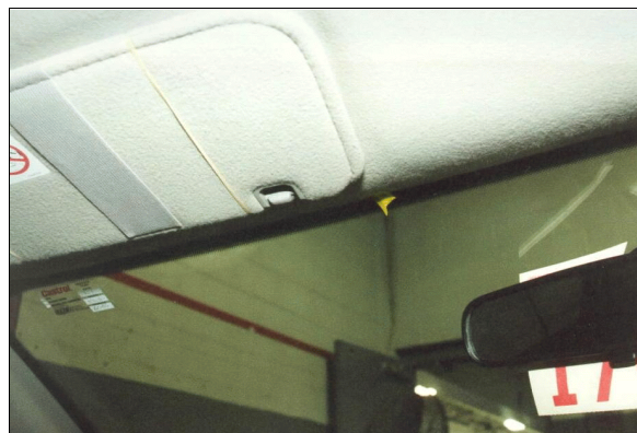
Figure 10: Possible contact evidence (i.e., yellow tape) on windshield header next to driver's sun visor (case photo #22)
