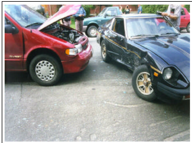
Figure 2. Damage and final rest positions.
