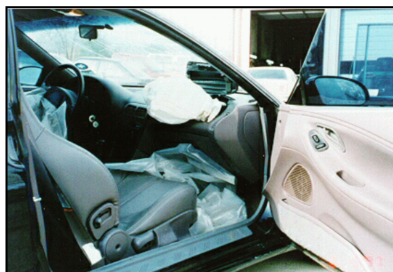
Figure 6: Case vehicle's front right seating area showing deployed front air bags and interior surface of right front door (case photo #12)
