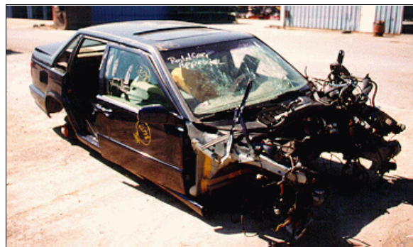
Figure 2: Case vehicle's damaged front viewed from right of front; Note: engine, wheels, etc. have been removed for salvage as well as missing crash damaged components (case photo #14)
