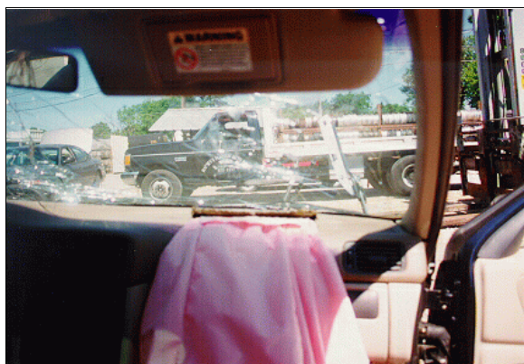
Figure 7: Case vehicle's deployed front right air bag and greenhouse area; Note: cracked right windshield directly corresponds to module's cover flap and sun visor is down in this photo but was most likely up at time of crash (case photo #26)
