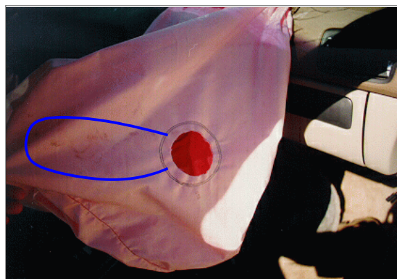
Figure 8: Close-up of case vehicle's deployed front right passenger air bag showing a vent hole and marks (highlighted) on underneath surface of air bag that are of unknown origin (case photo #29)
