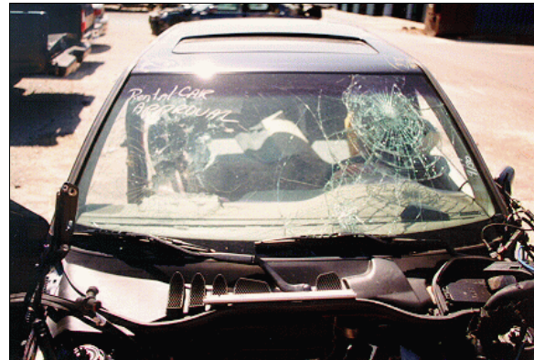
Figure 9: Case vehicle's cracked windshield; Note: spider web on driver's side indicates that the driver contacted the windshield while the crack on the passenger's side is from the air bag module's cover flap (case photo #02)
