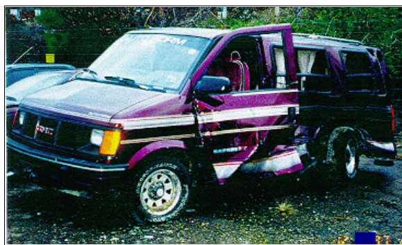
Figure 3: GMC minivan's left side damage viewed from left of front (case photo #34)
