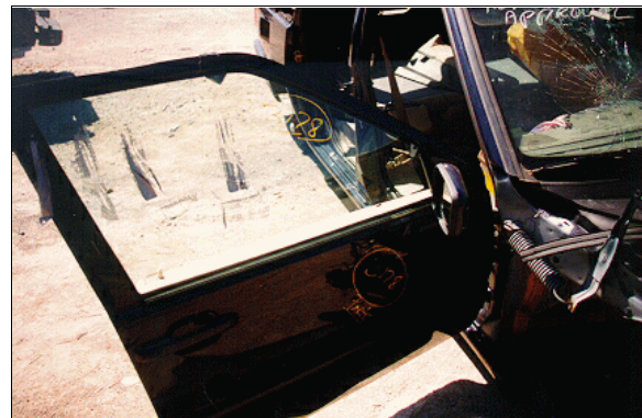
Figure 11: Case vehicle's right front window showing vertical marks on interior surface of glazing (case photo #15)
