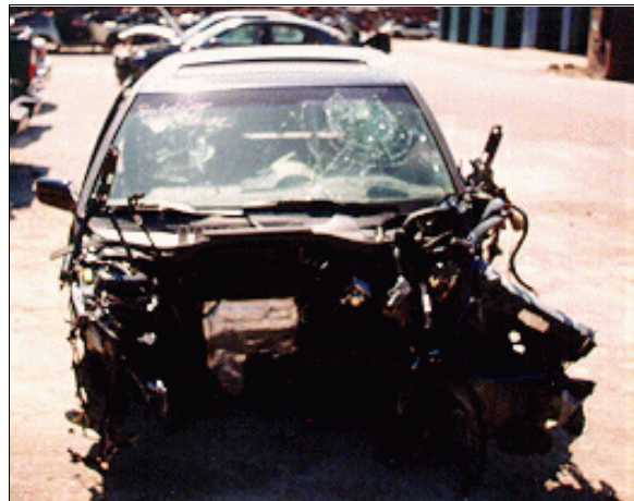
Figure 1: Case vehicle's damaged front; Note: damaged components have been removed and engine removed during salvage (case photo #01)
