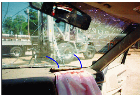
Figure 5: Case vehicle's front right air bag which deployed from the top of the right dash/instrument panel; Note: the right windshield was cracked by the air bag module's cover flap (case photo #21)
