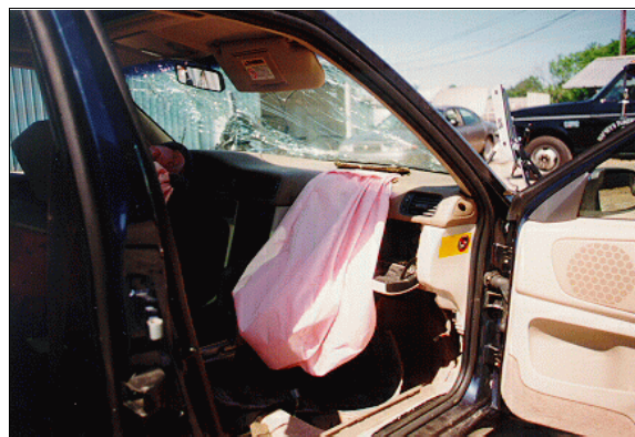
Figure 6: Case vehicle's deployed front right passenger air bag showing approximate size and shape of air bag's fabric (case photo #28)
