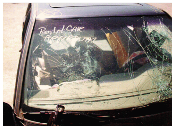
Figure 10: Close-up of case vehicle's windshield damage showing front right air bag module's cover flap lining up with cracked windshield; Note: driver's side appears to have two contact points, one near the header from the driver and one near the base from an unidentified source (case photo #16)
