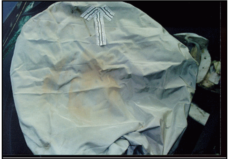
Figure 11. Interior, Vehicle 2. Shows make-up transfer from driver.
