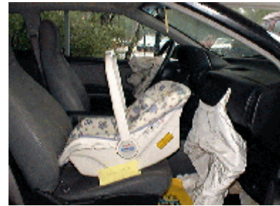
Figure 10. Profile view of the deployed front right air bag and the rear-facing child safety seat. (Seat track adjusted to the full rear position).
