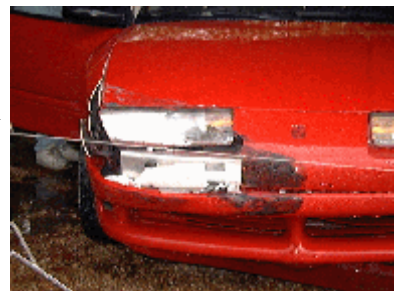
Figure 5. Frontal damage to the Saturn SC1.
