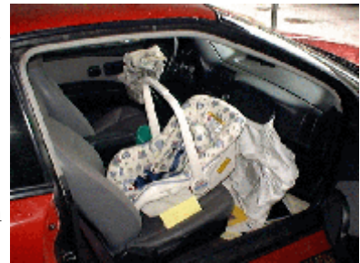
Figure 7. Overall view of the deployed mid mount front right air bag and the child safety seat.
