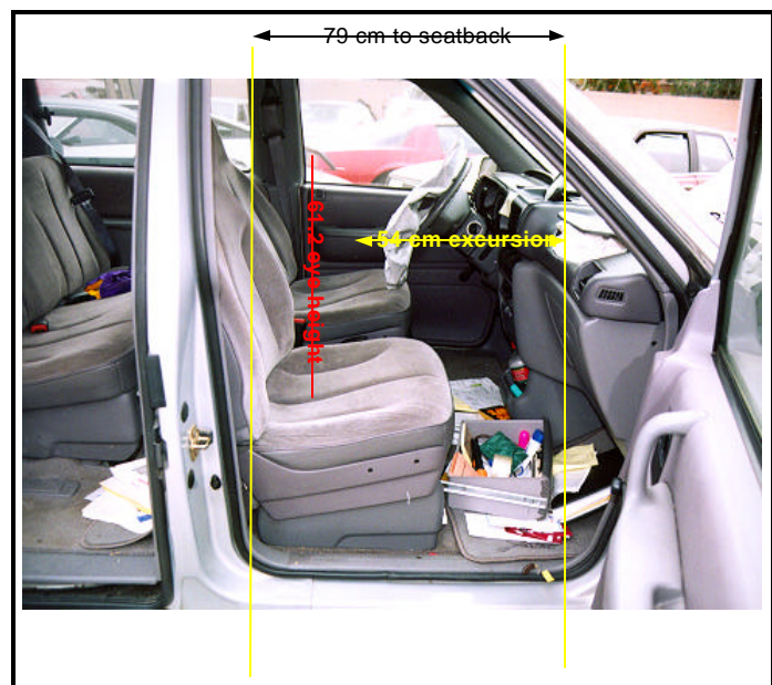
Figure 11. Interior, right side
