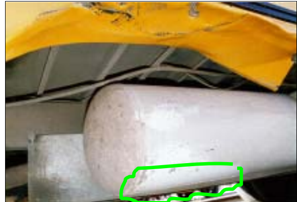
Figure 18: Close-up of GMC school bus's LPG gas cylinder under left body panel showing scrapes and yellow paint transfers (highlighted) to underneath side (case photo #59)
