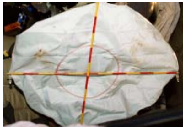
Figure 14: Case vehicle's driver (front) air bag showing blood on upper left quadrant and body fluids on upper right quadrant (case photo #35)
