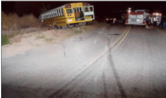
Figure 7: On-scene view looking south at tire marks and pavement gouges from both vehicles traveling to their final rest positions (case photo #75)
