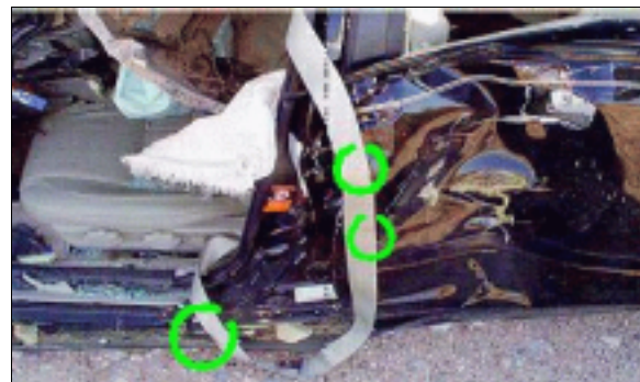
Figure 16: Close-up of case vehicle's left side impact showing driver's deployed seat back-mounted side impact air bag protruding from seat cushion and extended safety belt with blood spots highlighted on webbing (case photo #28)
