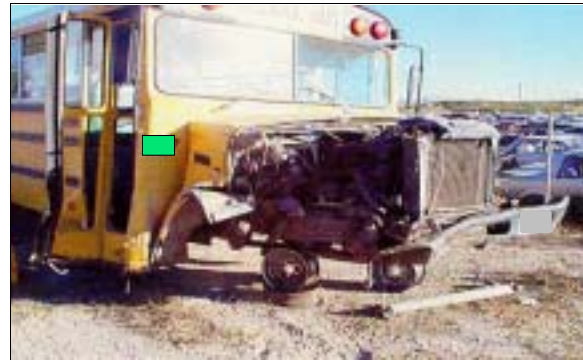
Figure 6: GMC school bus's frontal damage; Note: front axle and wheels were torn away, front shift, and side slap damage to folding entrance/exit door (case photo #72)
