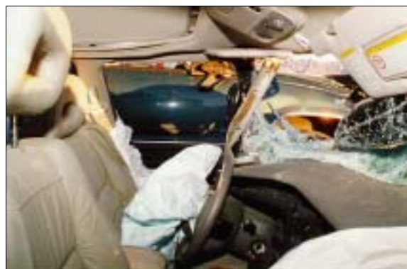
Figure 10: Case vehicle's front seating area viewed from right front passenger door; Note: extensive intrusion into driver's seating area (case photo #29)
