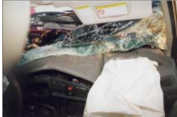
Figure 12: Case vehicle’s front right seating area showing deployed front right passenger air bag and extensive intrusion front instrument panel (case photo #34)
