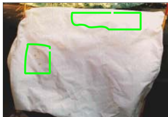
Figure 15: Front surface of case vehicle's front right passenger air bag showing blood evidence to left side and punctures along top (case photo #40)
