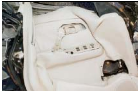
Figure 11: Interior surface of case vehicle's driver door showing extensive deformity (case photo #26)
