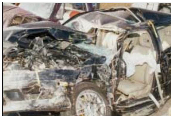
Figure 9: Case vehicle's extensive left side damage from impact with school bus; Note: yellow tape between left front bumper and "B"-pillar marks direct damage area (case photo #17)
