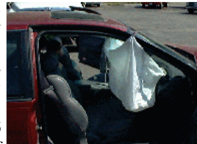
Figure 11. Deployed front passenger air bag.
