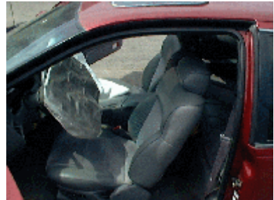
Figure 10. Profile view of the deployed front driver air bag.
