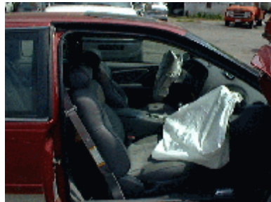
Figure 2. Profile view of the child passenger's position and the deployed air bag.
