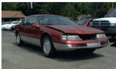
Figure 5. Front right view of the impact damage.
