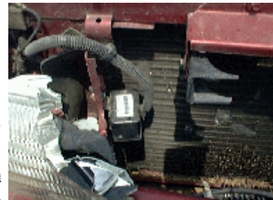
Figure 9. Rotated right crash sensor.
