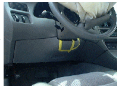
Figure 8. Driver knee contacts to the bolster.
