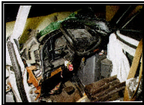
Figure 7: View of the steering wheel rim deformation.
