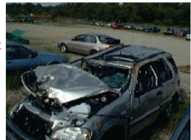
Figure 9. Left front three-quarter view of the rollover damage.
