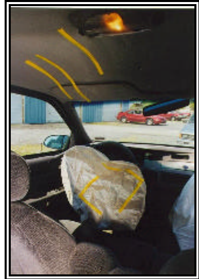
Figure 9. Vertical and rearward displacement of the child driver.
