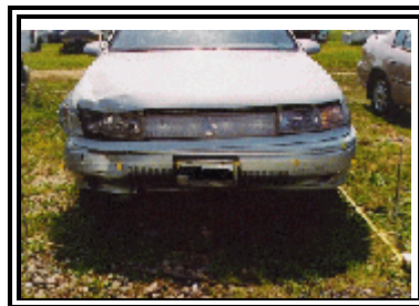
Figure 2. Front right damage resulting from the tree impact.
