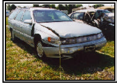
Figure 5. Damage to the front right area of the Sable.
