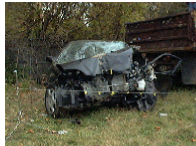
Figure 2. Frontal view of the impact damage to the 1998 Honda Civic.
