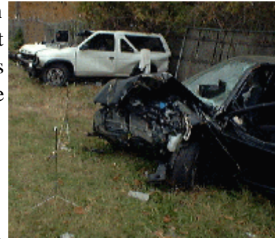
Figure 3. Profile view of the vehicle's damage pattern.
