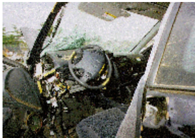
Figure 7. Interior damage/driver loading of the steering wheel.
