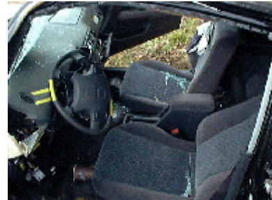
Figure 8. Non-deployed air bag and driver loading of the steering assembly.
