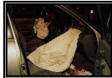
Figure 8. Deployed front right passenger air abg.
