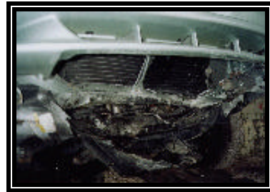
Figure 6. Radiator and crossmember damage from the curbed median.
