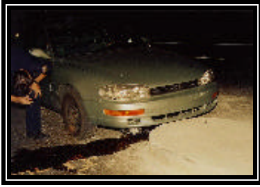
Figure 4. Lower front bumper fascia alignment with struck curbed median.
