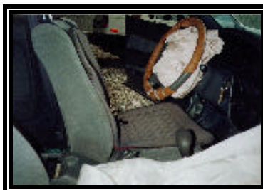
Figure 1. Forward seated position of the short stature female driver.
