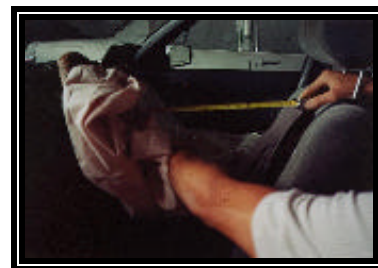
Figure 9. Police measurement of horizontal distance between the driver air bag module and the seat back.
