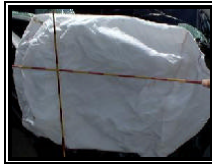
Figure 7. 1998 Chevrolet S-10 deployed redesigned passenger air bag.
