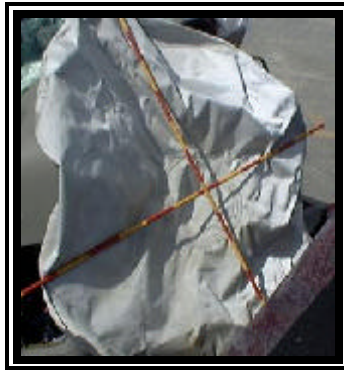
Figure 6. 1998 Chevrolet S-10 deployed redesigned driver air bag.
