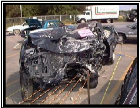
Figure 3. Frontal damage to the 1998 Chevrolet S-10 pickup truck.
