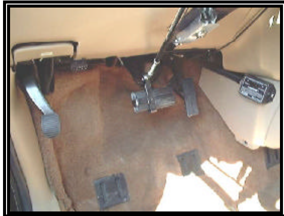
Figure 6: Close-up view of the mechanical brake actuation rod.
