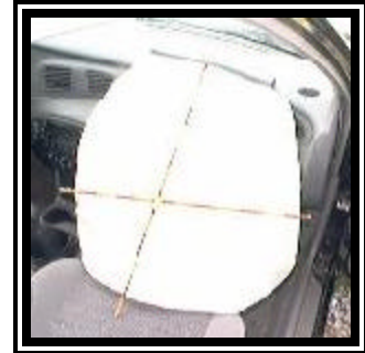
Figure 5. 1999 Ford Escort SE redesigned passenger air bag.
