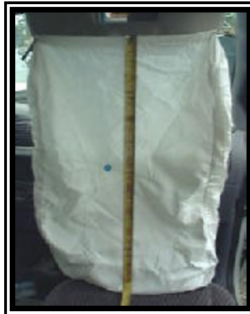
Figure 7. 1998 Dodge Caravan SE deployed redesigned passenger air bag.
