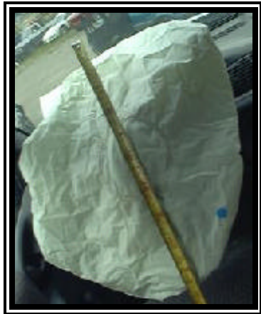
Figure 6. 1998 Dodge Caravan SE deployed redesigned driver air bag.
