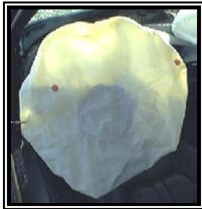
Figure 5. 1999 Dodge Stratus ES deployed redesigned driver air bag.
