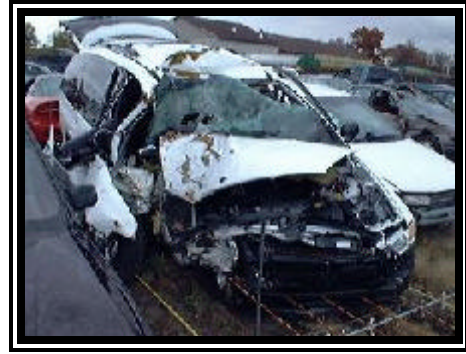
Figure 3. Front right damage to the 1999 Dodge Grand Caravan.
