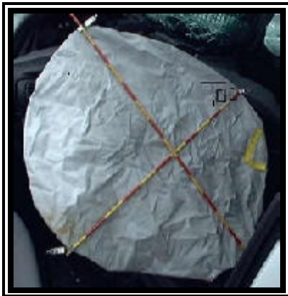
Figure 5. 1999 Dodge Grand Caravan deployed redesigned driver air bag.
