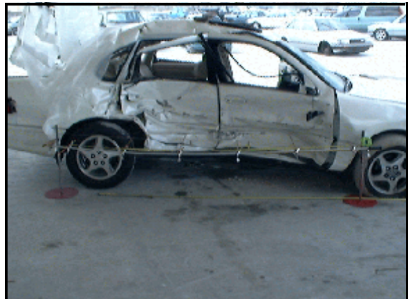
Figure 5: Case vehicle's right side damage from contact with vehicle #2
