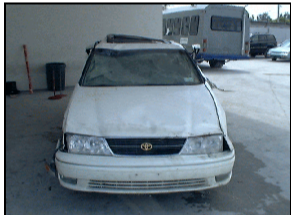
Figure 6: Case vehicle's damage from rollover; Note: front header and sunroof distortion
