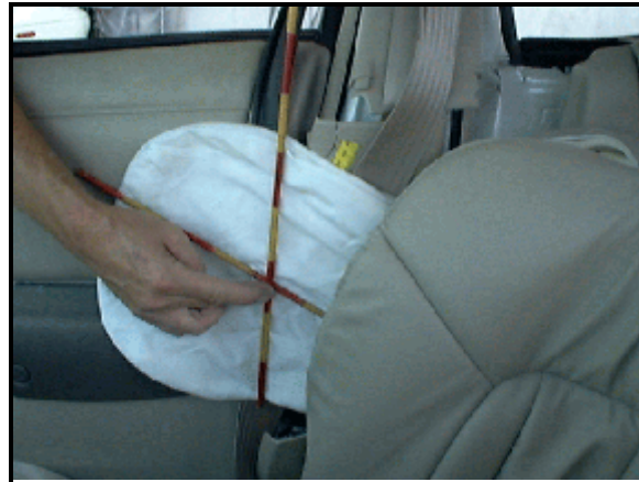
Figure 9: Case vehicle’s deployed front right passenger side air bag; Note: deformation to B-pillar’s vinyl cover
