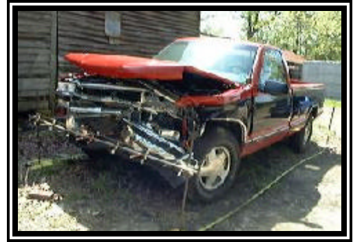
Figure 3. Front left damage to the 1998 Chevrolet C-1500 pickup truck.
