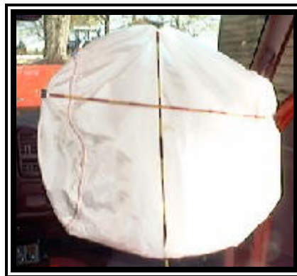
Figure 6. 1998 Chevrolet C-1500 pickup truck deployed redesigned passenger air bag.
