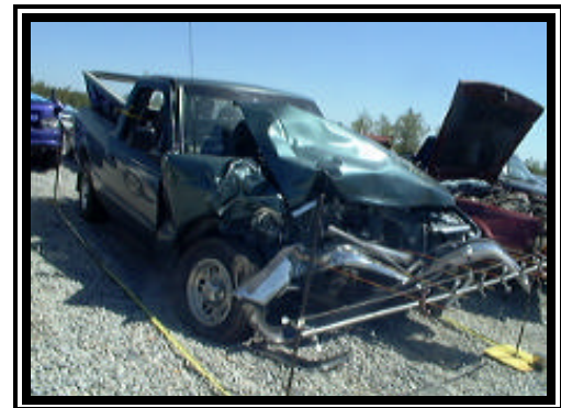
Figure 4. Front right damage to the 1995 Ford Ranger pickup truck.
