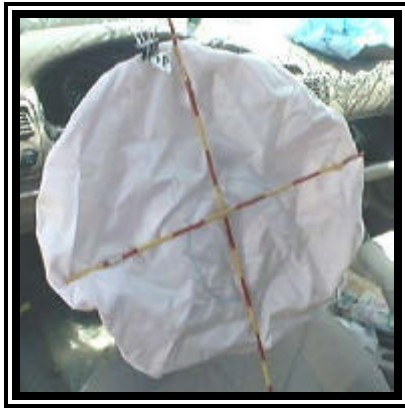
Figure 5. 1998 Toyota Corolla VE deployed redesigned driver air bag.
