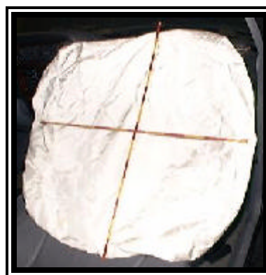
Figure 8. 1998 Jeep Cherokee Limited deployed redesigned passenger air bag.
