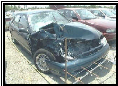
Figure 3. Front right damage to the 1998 Toyota Corolla VE.
