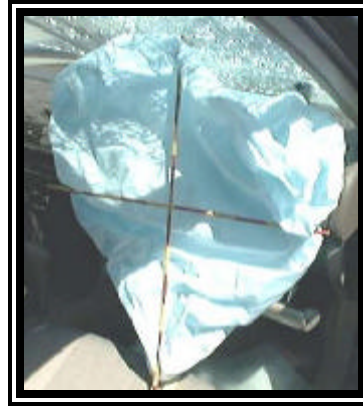
Figure 6. 1998 Toyota Corolla VE deployed redesigned passenger air bag.
