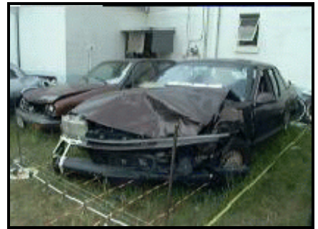
Figure 3. Frontal damage to Vehicle 1 (1989 Mercury Sable)
