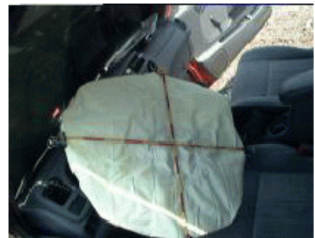
Figure 8. View showing deployed driver's air bag
