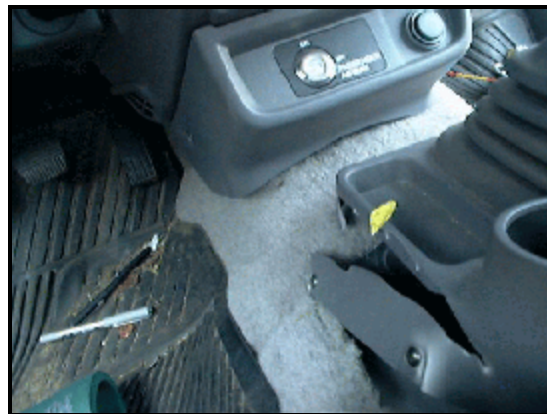
Figure 13. Close up view showing damaged center console due to right leg contact. Note: air bag shut off switch in off position
