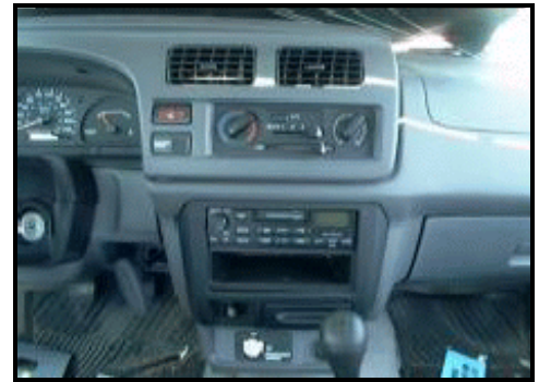
Figure 11. View showing air bag shut off switch
