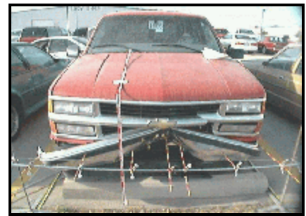
Figure 3. View showing frontal damage to Vehicle 2 (1999 Blazer)
