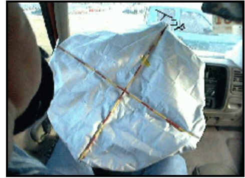
Figure 9. View showing deployed driver's air bag
