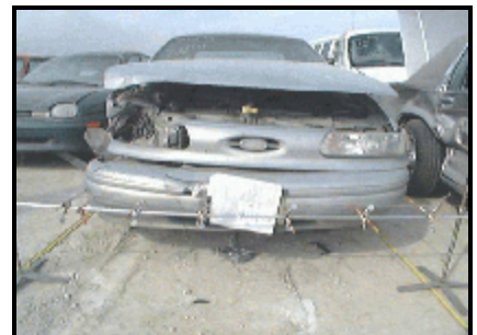
Figure 4. View showing frontal damage to Vehicle 1 (1994 Taurus)
