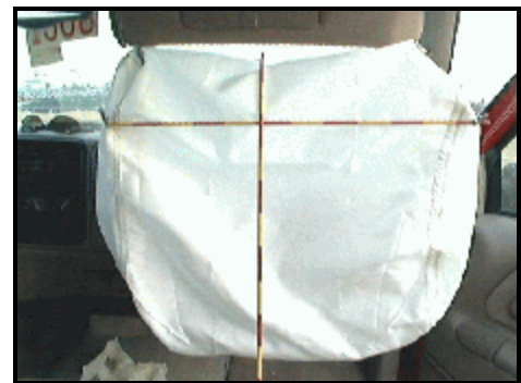
Figure 10. View showing deployed passenger air bag
