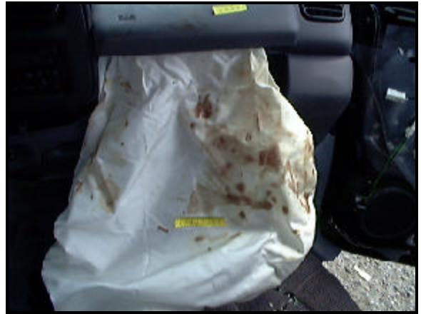
Figure 7. Passenger's air bag contact evidence.
