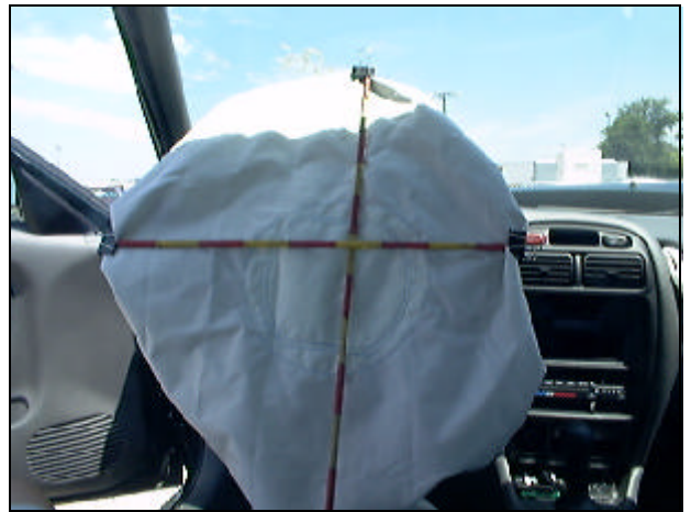
Figure 6. Interior, case vehicle. Driver's frontal air bag.
