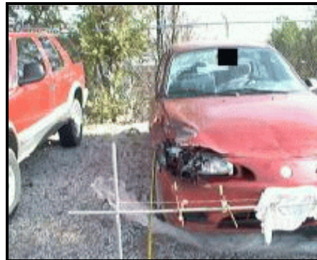
Figure 6. Front right corner damage to Vehicle 2
