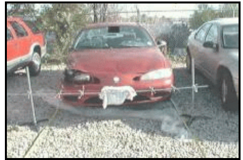
Figure 4. Front right corner damage to Vehicle 2 (Mercury Tracer)
