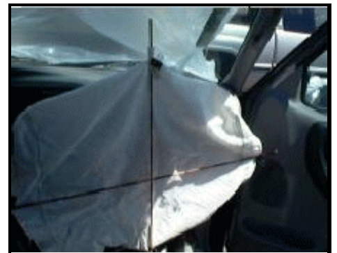
Figure 8. Passenger front air bag, Vehicle 1
