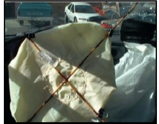
Figure 9. View showing deployed driver's air bag, Vehicle 2
