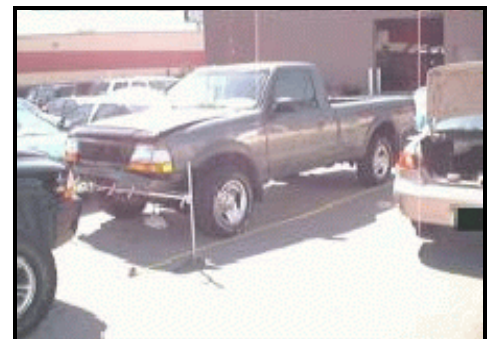
Figure 3. Frontal damage to Vehicle 1 (Ford Ranger)
