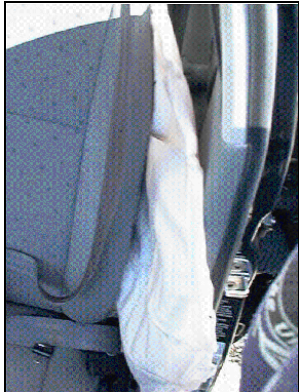
Figure 5: Deployed driver's seat back-mounted side air bag, looking rearward
