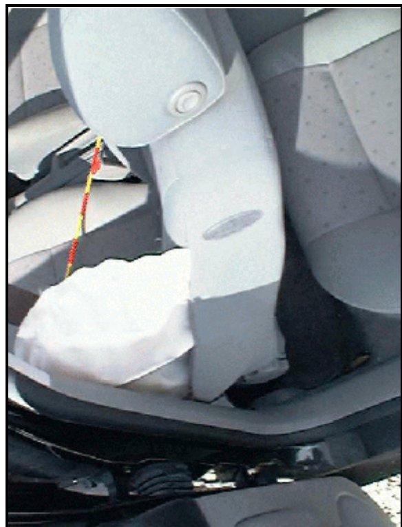
Figure 6: Looking down on deployed driver's seat back-mounted side air bag
