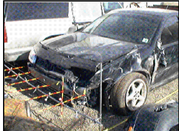
Figure 3: Front left view of damage to Jetta's front left corner from impact with embankment, which extended down left side
