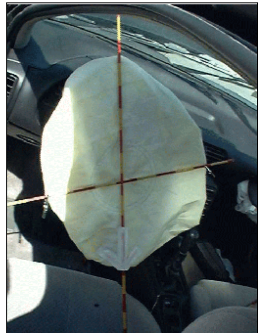
Figure 5. Deployed driver's frontal air bag
