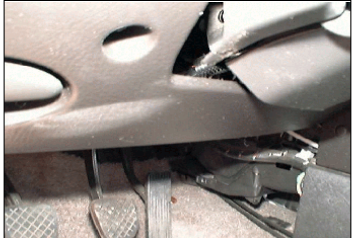
Figure 8. Contact mark to left instrument panel area
