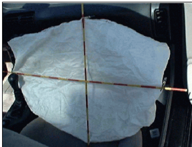
Figure 7. Deployed passenger's frontal air bag
