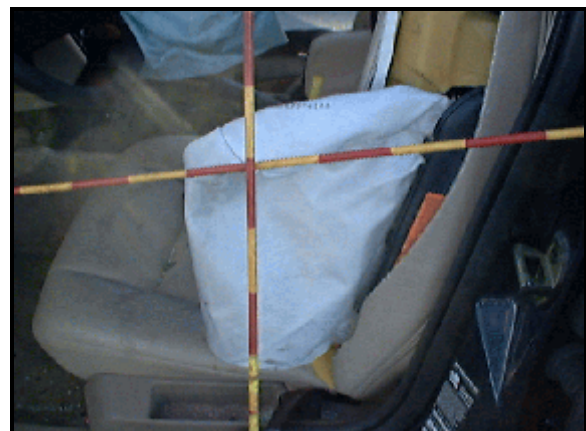
Figure 8: Driver's deployed side air bag
