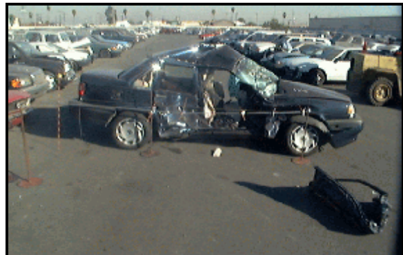
Figure 3: Case vehicle's right side damage; note, right front door in foreground
