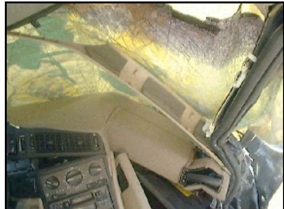
Figure 7: Non-deployed front right passenger's air bag module cover
