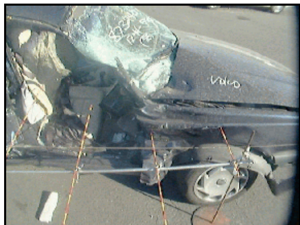
Figure 4: Case vehicle's front right seat position; note, relatively undamaged seat cushion
